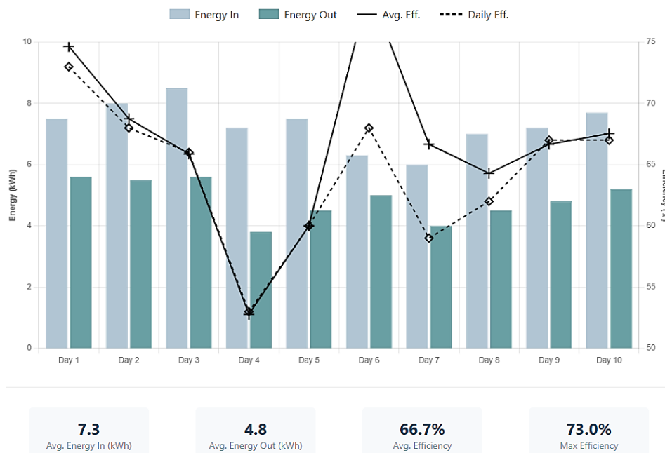
Figure 3 Measured energy output and efficiency of a hybrid solar–wind microgrid over 10 days (Muhuru Bay, Kenya).
