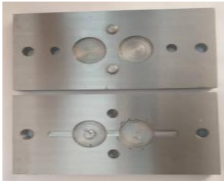
Figure 2. The fabricated mould.
