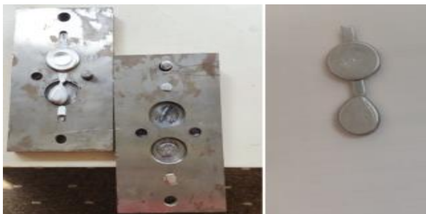
Figure 3. Pouring without preheat the mold (incomplete filling).
